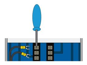
**11.** Slide the U connectors for Sector 1 sector run under the square washer at the input terminal. See Figures C, D & E.
