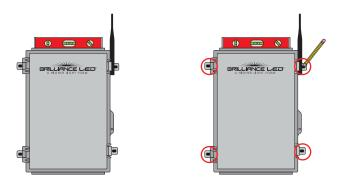
**4.** Use a 1/4" drill bit for the pilot holes. Use the Mounting Anchors and Screws provided to mount the Sector Selector to the surface.
