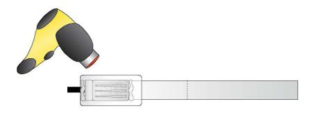
**12.** Connection is now complete. Allow any additional silicone to squeeze out, and wipe off the excess.
